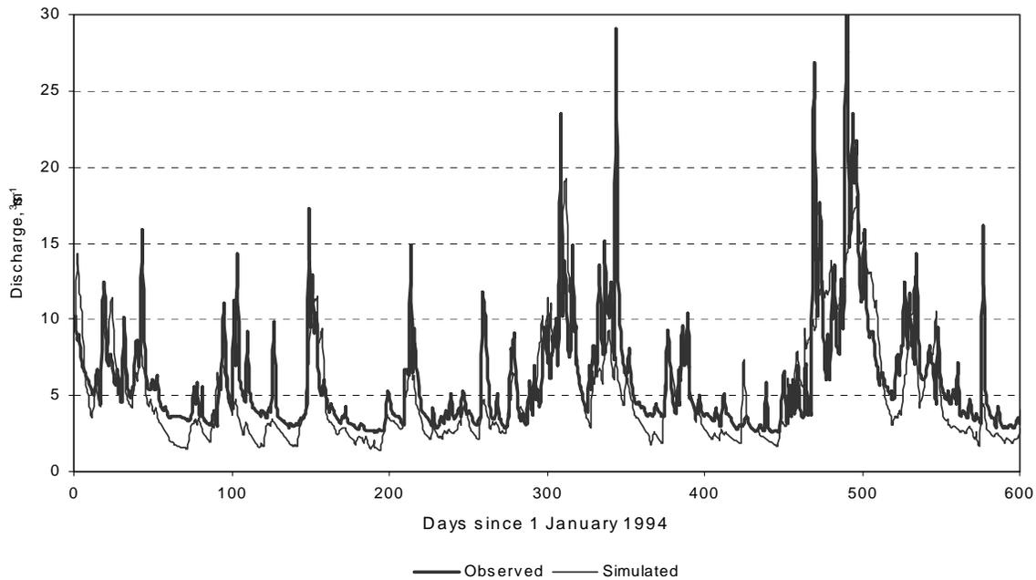
Fig. 7 : The extracts from observed and simulated by FDC method daily flow time series for Rakwana Oya at Thimbolketiya.
